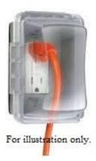
**8.07 Ground Fault Circuit Interrupters** - The purpose of a GFCI is to provide protection against shock hazards. It will open or "trip" on slight imbalances in current flow, thus protecting you. The GFCI operates as other circuit breakers, should it "trip," simply reset it for continuing operation. Periodically, you should test the GFCI for proper operation. By pushing the test button, the GFCI should trip to the "OFF" position.
